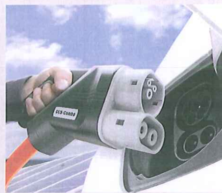
Ionity CCS (Combined Charging System) Combo
